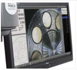
'Next generation' measurement software coupled with a high resolution video camera enables Falcon to measure a wide variety of simple and complex features, quickly and simply. Essential measurement data, with graphics-based "part view" construction is displayed alongside the high resolution video image.
