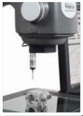
A touch probe option provides non-contact and contact measurement in a single system, allowing fast and repeatable measurements in the Z-axis.
